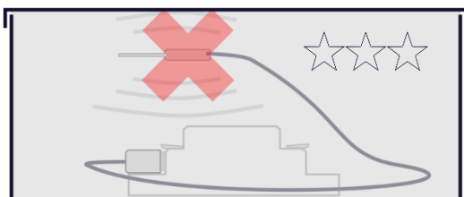
Figure 4: Do not place the antenna in a metal housing / junction box.
