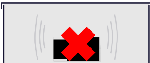
Figure 5: Do not place the micro BLC industrial 4 channel in a metal housing / junction box.
