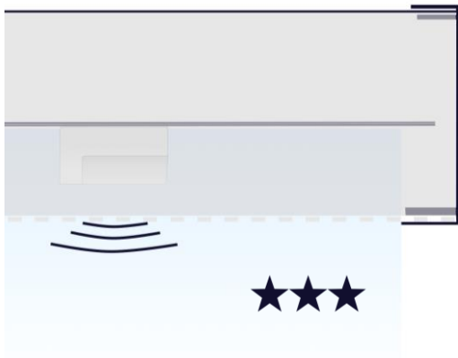
Figure 3 : In case of a metal fixture place the Micro BLC on the side of the light diffuser.
