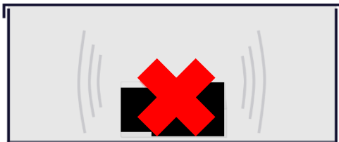
Figure 5: Do not place the micro BLC industrial DALI in a metal housing / junction box.
