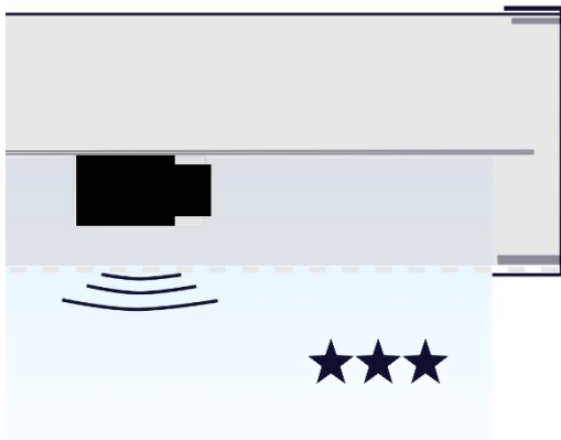
Figure 3: In case of a metal fixture place the micro BLC industrial DALI on the side of the light diffuser.
