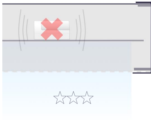
Figure 1: Do not place the Micro BLC in a metal housing / fixture.
