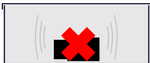
Figure 5: Do not place the micro BLC 0-10V industrial in a metal housing / junction box.
