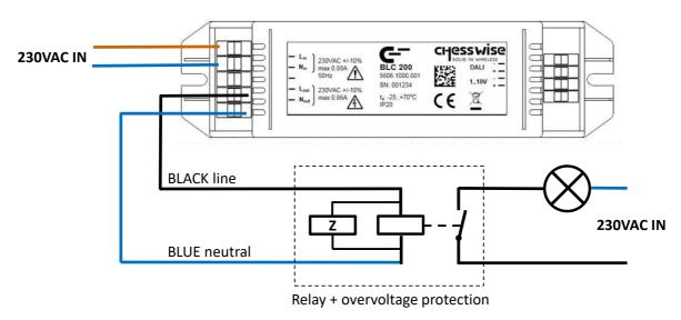
Connect the external 230VAC relay + overvoltage protection to the switched 230V output of the BLC200.
