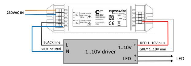
Connect the power input of a 1..10V driver to the switched 230V output of the BLC200.
