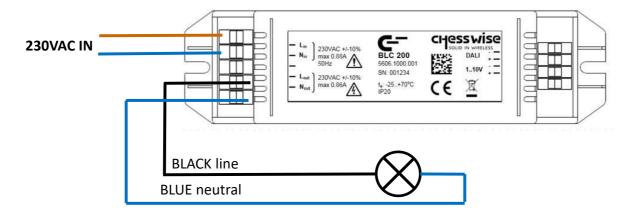
Connect the 230V load to the switched 230V output of the BLC200
