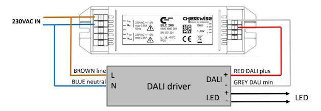
Connect the power input of a DALI driver directly to the 230V mains.
