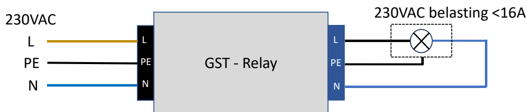
GST-Relay + 230VAC belasting
